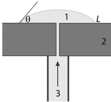
FIGURE 10. Schematic illustration of the formation of a drop by appropriate liquid pumping.  $L$ -radius of the drop base;  $\theta$  - contact angle. 1- liquid drop, 2- solid substrate with a small orifice in the center, 3 - liquid source/sink (syringe).
