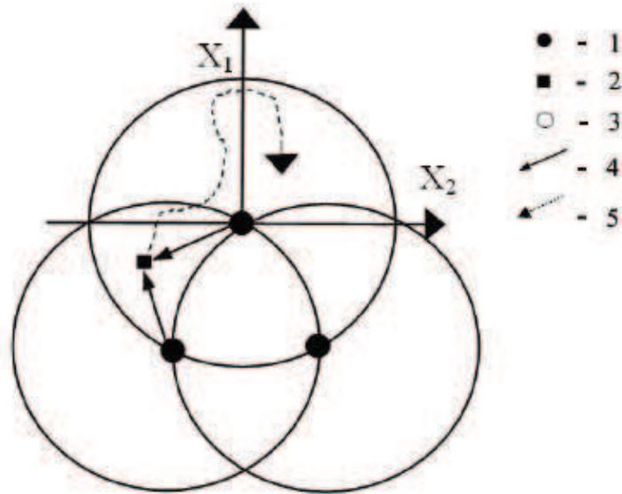
Figure 1: Schematic representation of the system's behaviour model: 1 – equilibrium state; 2 – object under study; 3 – layer of the space of states; 4 – deviation of characteristics of the object under study from equilibrium ones; 5 – trajectory of object movement
